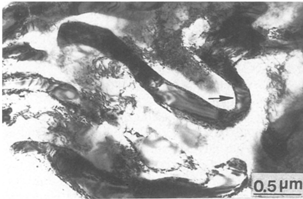
Figure 9 Kinking of cementite lamellae in a pearlite colony after 20% reduction (steel B).
